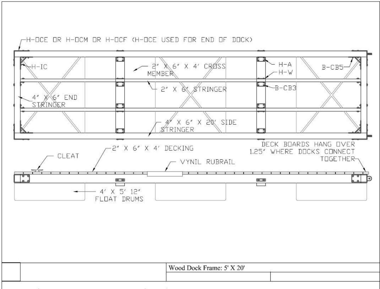
**Figure 2 Typical 5' x 20' Wooden Float (with encased buoyancy billets)**
